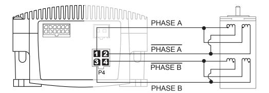
Figure 2.3.3: 8 Lead Motor Parallel Connections
